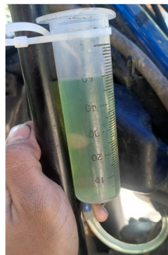
Figure 3. Measuring cylinder connected to the carburetor
