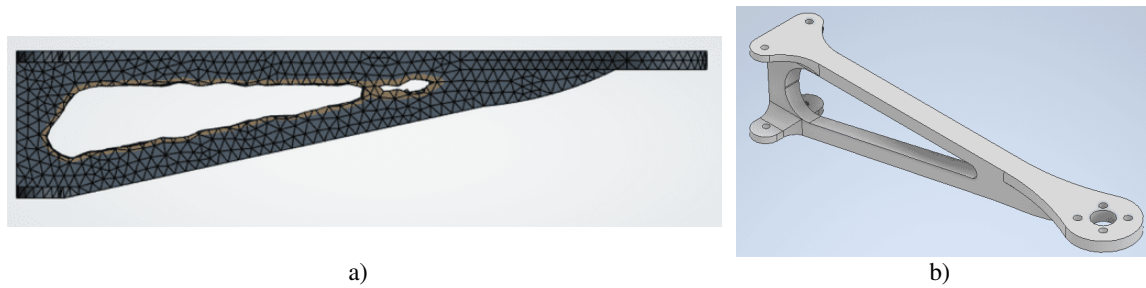
Figure 8. a) Topology optimization result, b) Final CAD design
