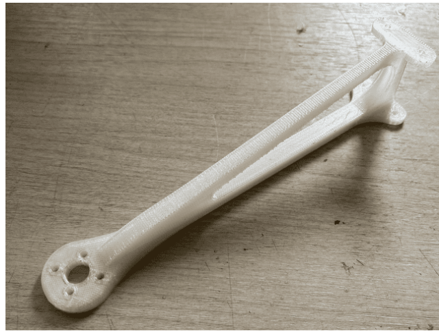
Figure 11. 3D-Printed result of the drone arm
