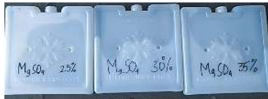
Figure3. PCM MgSO_4 with MgSO_4 25%, MgSO_4 30%, MgSO_4 35% composition
